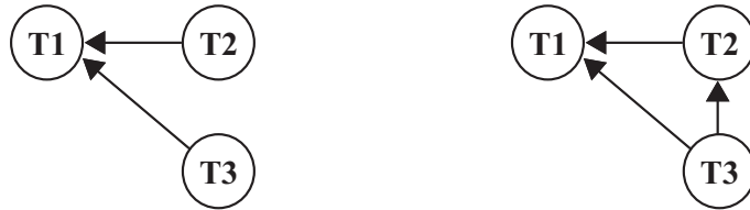
Figure 4.5: Waits-for graph of three transactions in the example. These edges represent the request to the region R . The left graph is invalid under LAS protocol. The right one exactly obeys LAS protocol.
